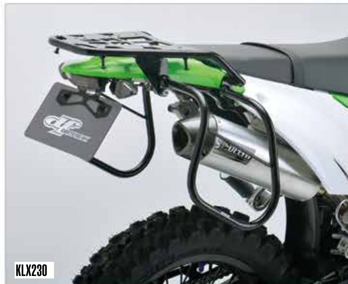
KAPPA saddle bag installation example
